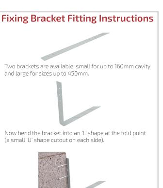
Once folded the bracket can be fixed to the block (or CP board). It is recommended to use at least two fixing points to ensure strength. Non-combustible fixings of appropriate type and strength for the substrate and application should be selected.
